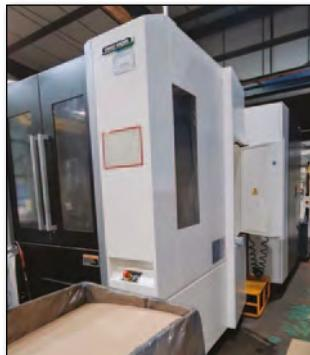
DMG MORI NH5000 DCG CNC Twin-Pallet Horizontal Machining Centre, F31iB CNC control, 500 x 500mm pallet, BT40 spindle, 14,000rpm spindle, through-spindle coolant, full 4th axis, 120-station ATC, tool brake check, swarf conveyor, Filtermist FX4002F mist extraction unit, Hydrael M530-1000 high pressure coolant system, Eclipse magnetic filtration, s/n NH503211202 (**2022**)
