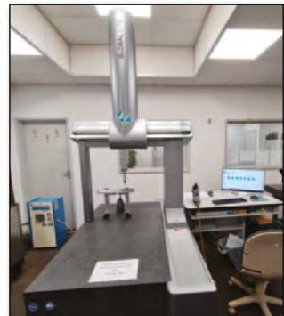
HEXAGON Metrology Global Lite CNC CMM, 1,650 x 850mm granite bed, 820mm between columns, Hexagon probe & holder with PC, software & HH-C-V2.1 control (**2022**)
